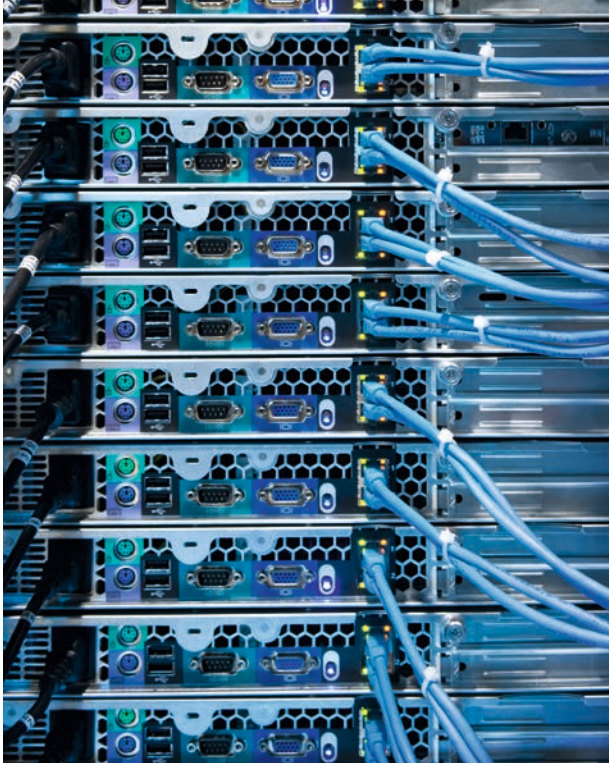
Modern high-performance data cables bring high-speed Internet into buildings. The coating of these data cables consists of ethylene and propylene.
